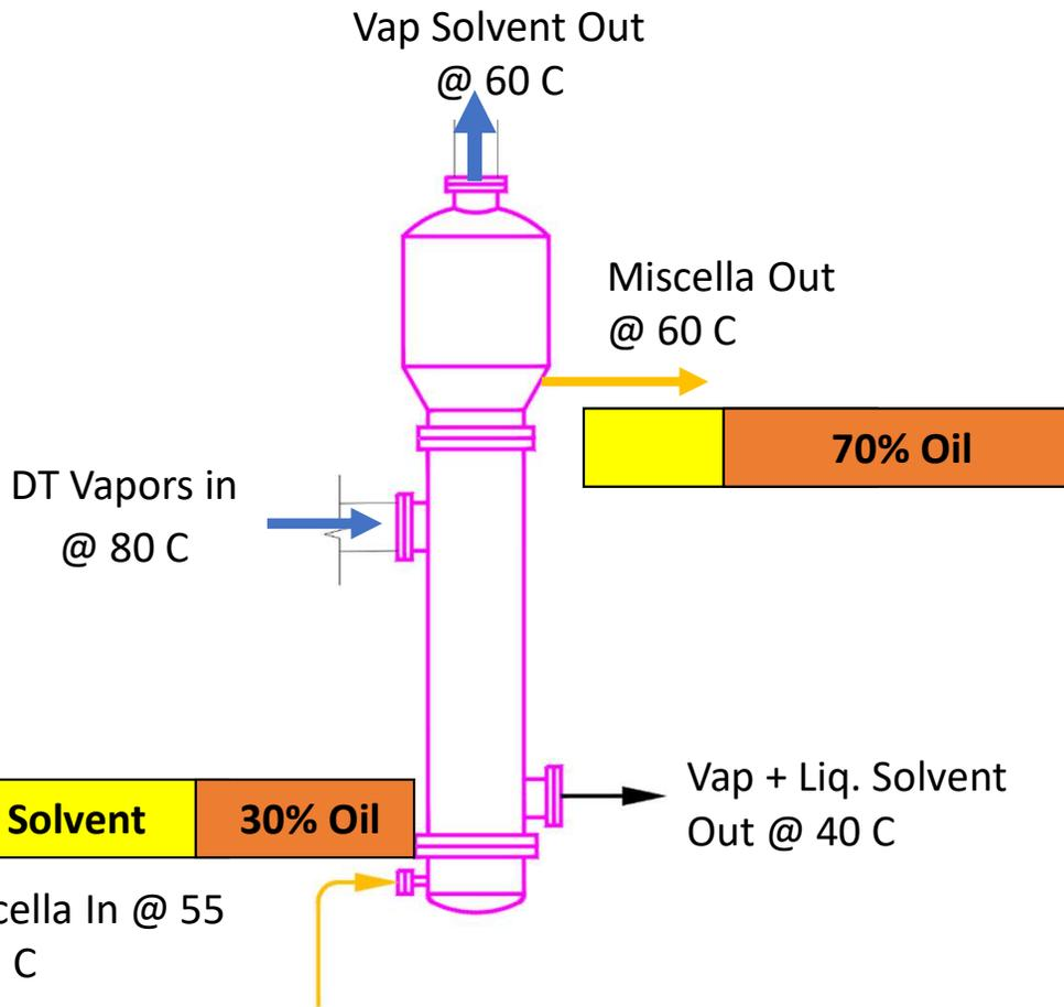
By using heat from DT vapors, we can vaporize around 75% of solvent present in incoming Miscella
