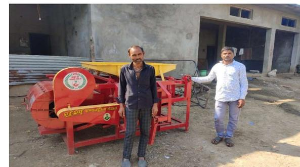
Multi grain Semi automatic Grader machine
