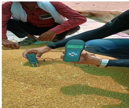
**Demo being given on Grain moisture meter**
